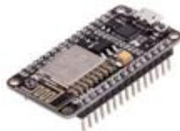
Fig 1.1 NodeMCU
